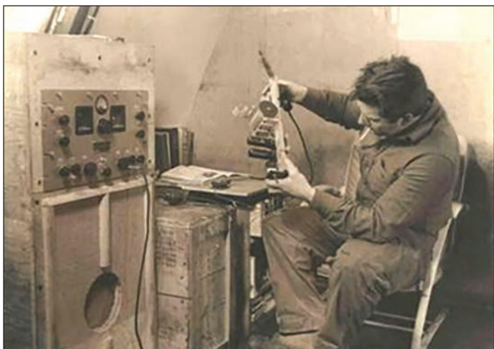
Figure 2: The 5 watt transmitter built by Chet Twombly from spare parts.
